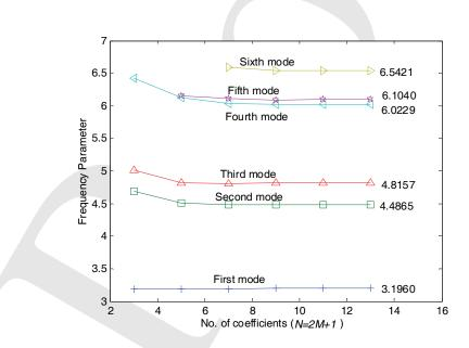
Figure 10: The lower six natural frequency parameters and mode shapes for a clamped circular plate containing three holes with free edge by using the present method, semi-analytical method and FEM
