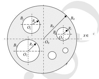
Figure 1: Problem statement for an eigenproblem of a circular plate with multiple circular holes
