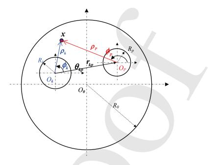
Figure 2: Notation of the Graf's addition theorem for Bessel functions
