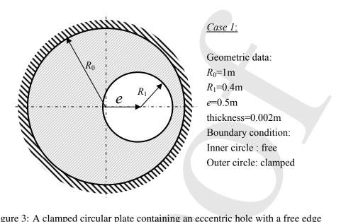
Figure 3: A clamped circular plate containing an eccentric hole with a free edge
