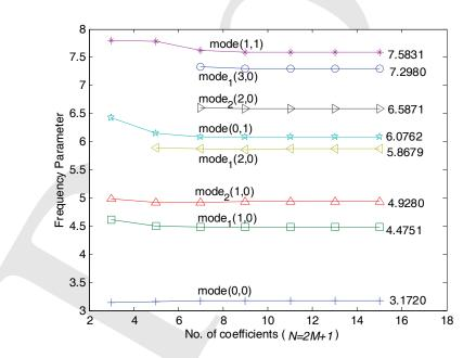
Figure 4: Natural frequency parameter versus the number of coefficients of the multipole representation for a clamped circular plate containing an eccentric hole with a free edge ( $R_0$ =1.0,  $R_1$ =0.4 and  $e/R_0$ =0.5)
