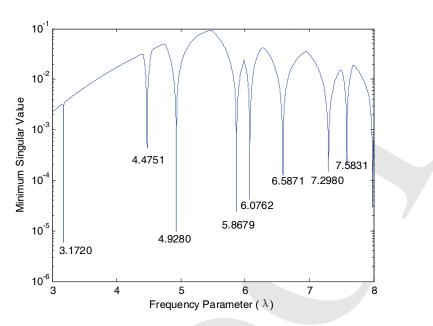
Figure 5: The minimum singular value versus the frequency parameter for a clamped circular plate containing an eccentric hole with a free edge ( $R_0$ =1.0,  $R_1$ =0.4 and  $e/R_0$ =0.5)
