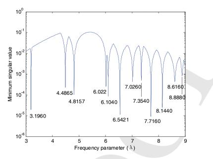
Figure 11: The minimum singular value versus the frequency parameter for a clamped circular plate containing three holes with free edges
